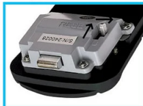
3. Set your favorite combination and push the lever to A
